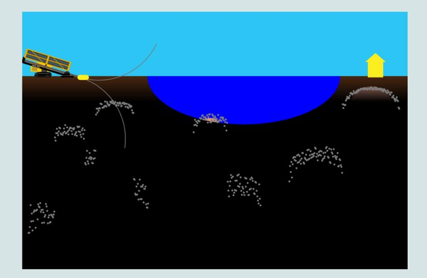
As you start drilling, the fog clears following the bit, simulating an LWD tool with a limited look around.
